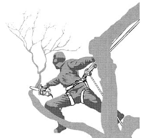
Figure B.5- Example of one-handed chain saw use
