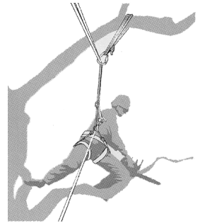
Figure B.3 - Example of redirection of main line via supplementary anchor point
